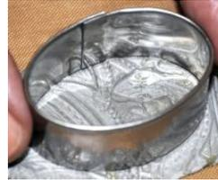
4) Cut out the general ring blank using a small oval cutter.
